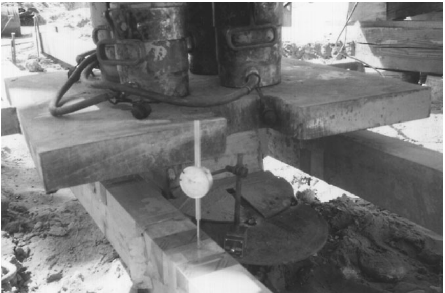
FIGURE 13.27 Pile load tests. This photograph shows one of the dial gauges that are used to record the vertical displacement of the top of the pile during testing.
