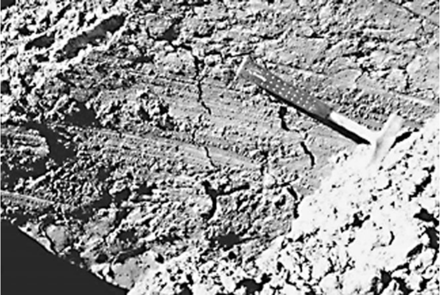
FIGURE 11.3 Close-up view of the fault plane. The striations indicate predominantly horizontal movement with some vertical movement. (Photograph from the Steinbrugge Collection, EERC, University of California, Berkeley.)
