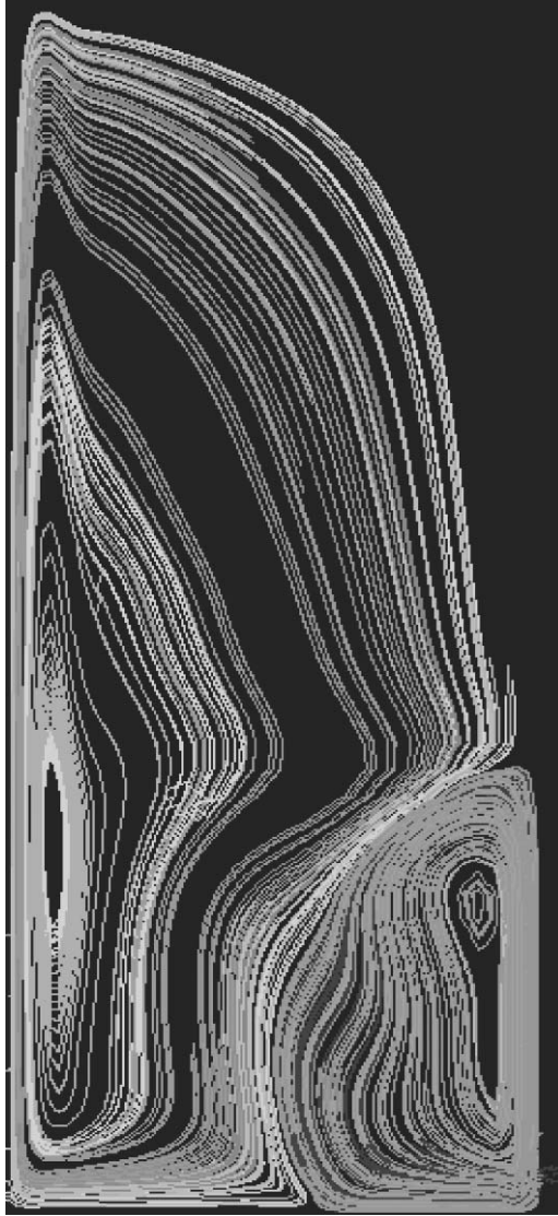
Figure 5.3. Flow patterns of water in a cylindrical can after 180 s of heating. The right-hand side of the figure is the centerline.
