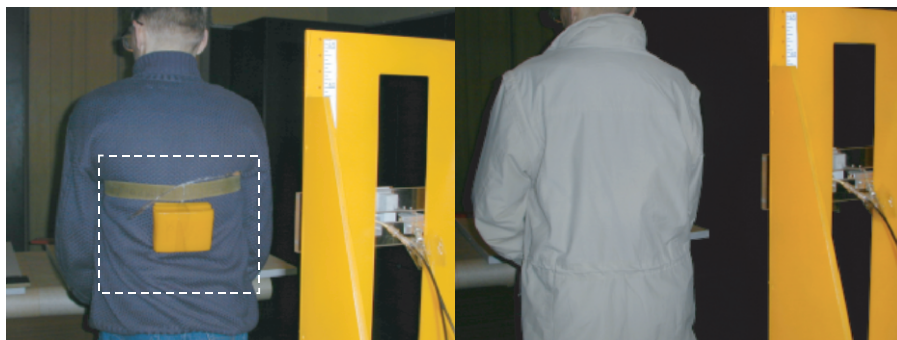
Figure 2. Experimental setup with two antennae. “Suicide bomb” was simulated by wax attached to the body and covered by a raincoat
