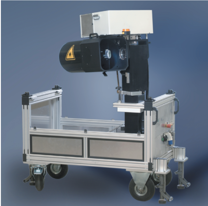
Figure 6. Photo of the transportable LSA TeleLis system. The total height is about 1.8 m
