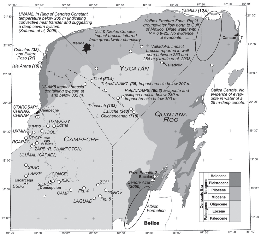
Figure 6.1: Sites of sampling. Source: Research data on the geology and hydrogeology of the Yucatan peninsula. Location of sampling sites for this paper in Campeche and southern Quintana Roo are shown. Also shown are specific aspects of the hydrogeology of the northern peninsula. Unless indicated, these summarize information in Perry et al. (2009). Numbers in parentheses within sample bullets are R values for water samples from lakes and municipal wells [ R = 100[(Sr)/(Cl)] in meq/kg].
