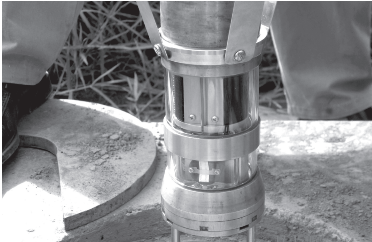
Figure 30.1: Camera used to record the interior of water supply wells. Source: By the authors.
