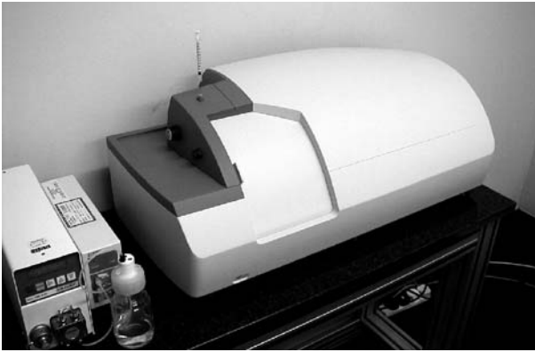
Fig. 16. DPI. A bench-top instrument for the study of protein structure in real time (Cross et al. 2004)
