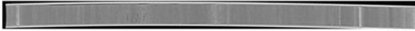
Fig. 20.7 Topogram (1.5 m long) reconstructed from 3750 overlapping tomograms. The image is in DICOM format; grey-level values correspond to hounsfield units
