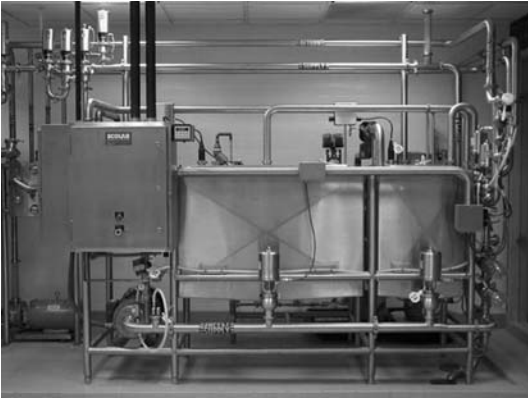
Figure 11-7 A CIP single-use solution recovery unit that is part of a system containing a water supply tank and CIP circulating unit. Courtesy of Ecolab, Inc., St. Paul, Minnesota.
