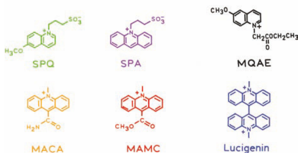
Figure 19.16. Representative chloride probes. These probes are collisionally quenched by chloride (Table 19.1). Revised and reprinted with permission from [49]. Copyright © 1994, Academic Press Inc.
