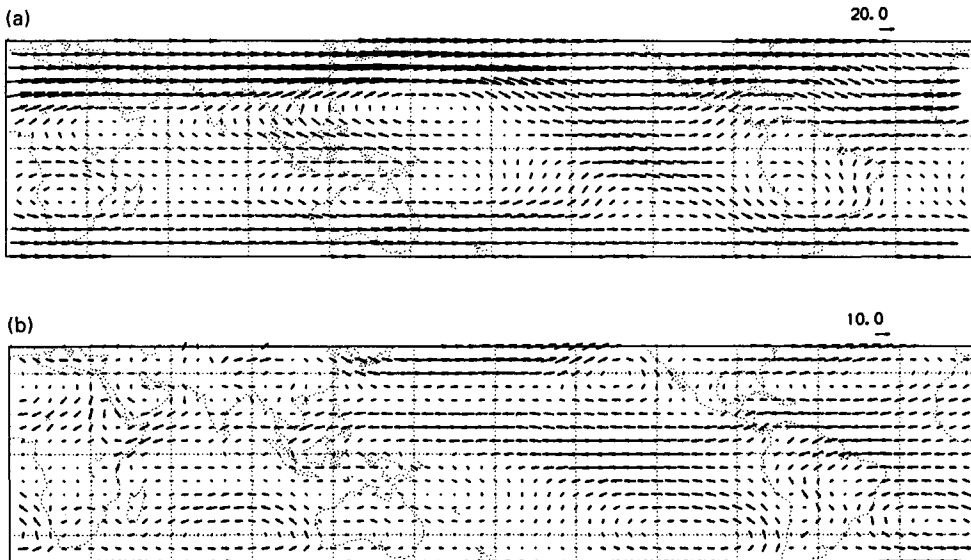
Fig. 7.1. Vectors of the time mean horizontal wind, \bar{v} , for the DJF season. Based on six years of ECMWF data for the DJF season. (a) At 15 kPa, near the tropical tropopause: the sample vector represents 20 \text{ m s}^{-1} . (b) At 85 kPa, just above the atmospheric boundary layer. The sample vector represents 10 \text{ m s}^{-1} .
