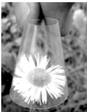
Fig. 11 High transparency of a BC nanocomposite demonstrated by the view on a flower through a corresponding foil. Reprinted with permission from [55]
