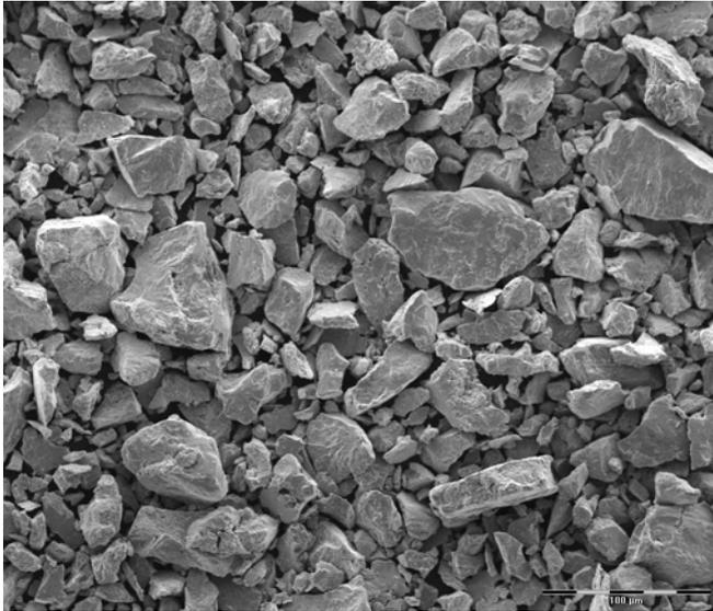
*Figure 1.* SEM micrograph of the Fe–Si investigated in the present experiment.
