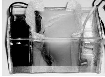
Figure 2. Appearance of a gel crack during electro-osmosis tests.
