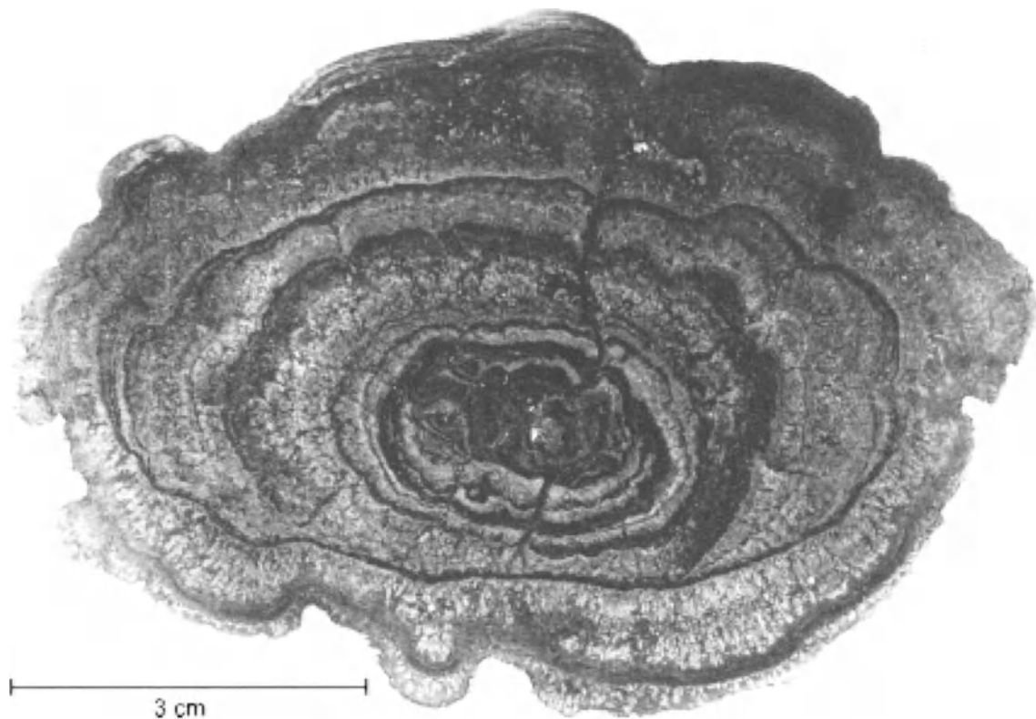
Fig. 11.10 Vertical section of a hamburger-shaped nodule from the Clarion-Clipperton F.Z. region displaying a layered growth structure (1 D s_r ). The nodule nucleus is a nodule fragment. Sample collected at Stn 178 GBH, R.V. Valdivia cruise VA 13/2 (9°22.5'N, 145°53.1'W, 5231 m). Photograph courtesy of U. von Stackelberg, BGR.
