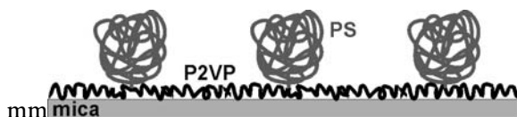
Fig. 1 Scheme of the structure of adsorbed PS- b -P2VP in ultra-thin films on mica. The P2VP adsorbs on the surface, whereas the PS dewets the adsorbed layer and forms isolated clusters
