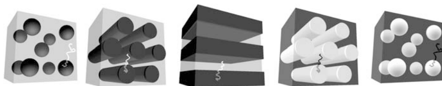
Fig. 11 The classical morphologies in block copolymer systems
