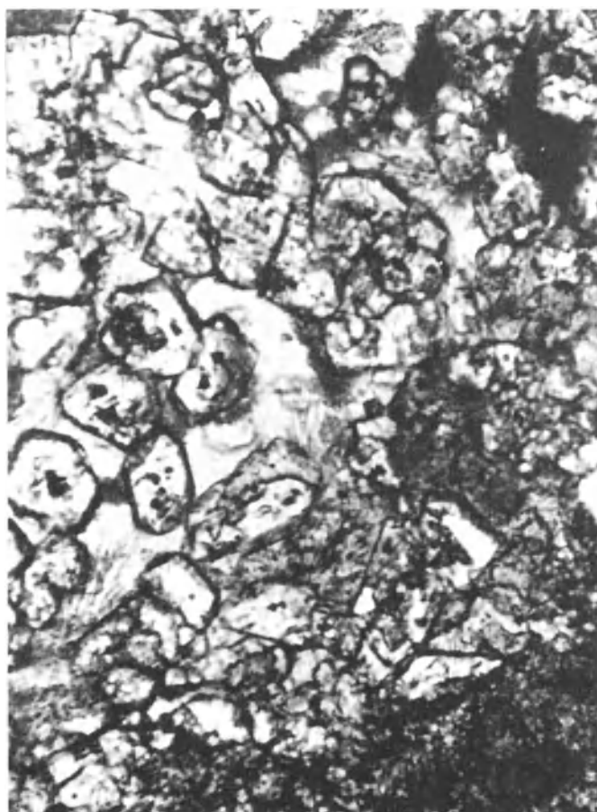
Fig. 3. Portion of an olivine crystal replaced by euhedral monticellite (high relief) and anorthite (low relief), pp. light, X225.
