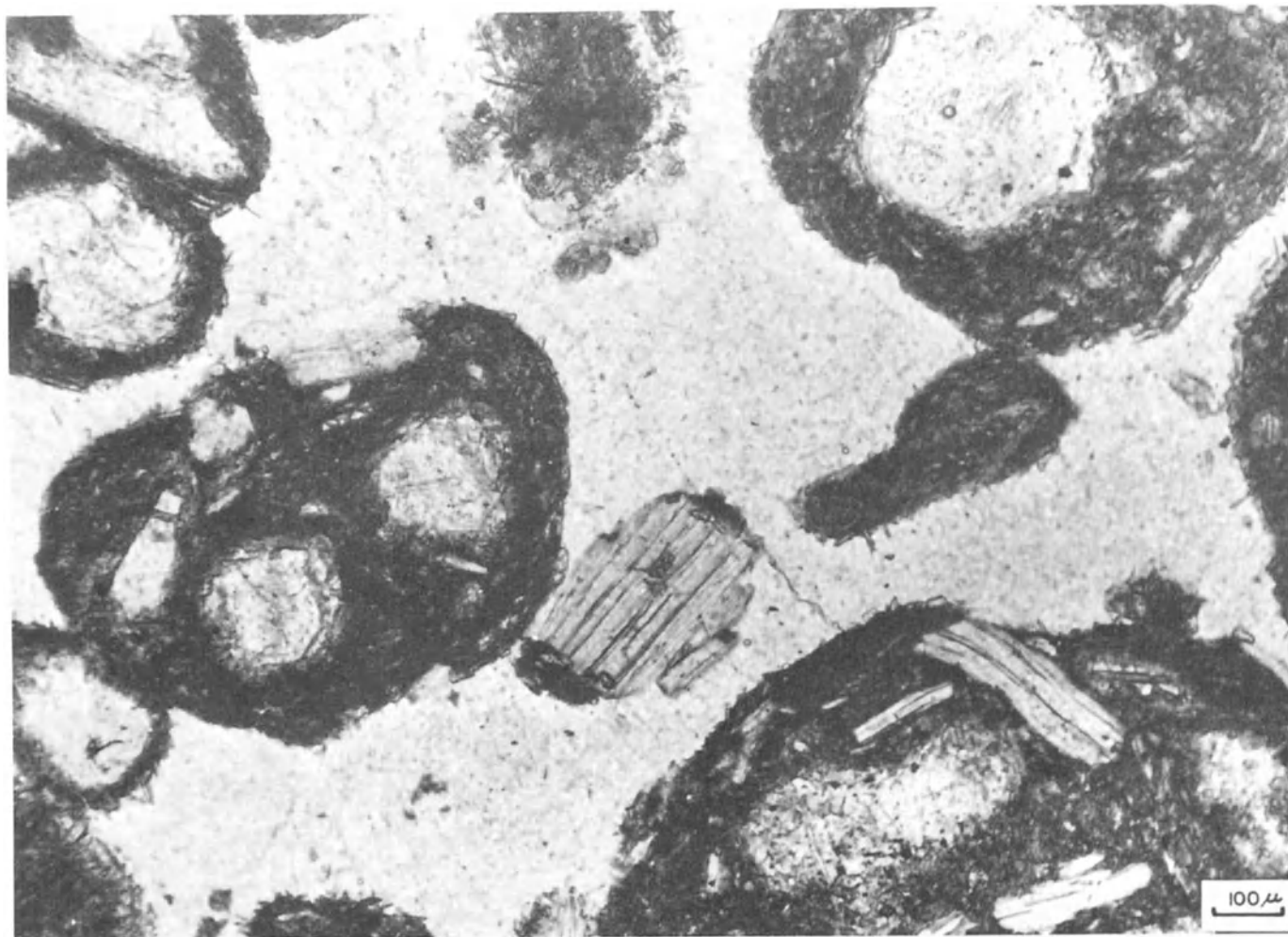
Fig. 3. A serpentine-phlogopite kimberlite, from the Finsch pipe. Globular segregations (autoliths) contain mainly phenocrysts of olivine (serpentinized) and phlogopite plus very fine-grained phlogopite and diopside. The interautolithitic material is essentially serpentine.
