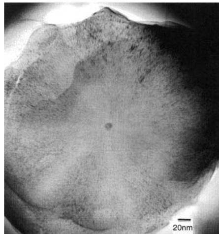
1(c) An onion from sample LFC1 with a central 10 nm TiC crystal (dark central spot) in a nanocrystalline core; the ‘radial spokes’ are due to a diffraction effect. The onions are spherules with a platy, continuous concentric layering of fairly well developed, parallel graphite (002) lattice fringes. Scale bar is 20 nm
