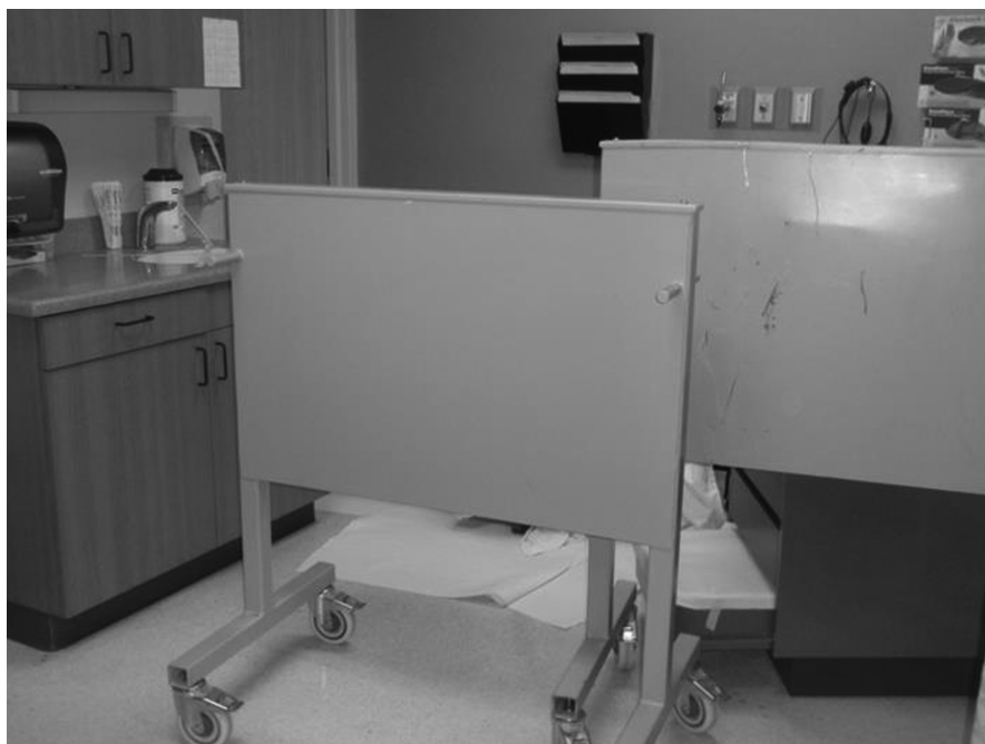
Figure 7.3 Bedside shields used to protect nurses and other patient-care staff from radioiodine gamma ray exposure during patient-care activities
