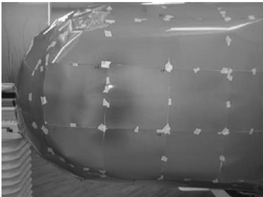
Figure 7.1 Radiochromic film taped to head of linear accelerator to monitor for leakage radiation
