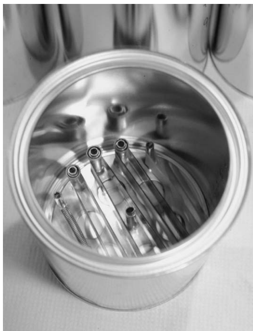
FIGURE 4.2 For storage and shipping, SPMDs (shown on a deployment apparatus rack) are placed in a clean metal can, flushed with argon, and sealed with a gas tight lid. This figure reproduced courtesy of the American Petroleum Institute (Huckins et al., 2002).
