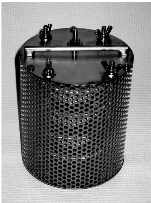
FIGURE 4.1 A stainless steel deployment device designed by Harry Prest, Santa Cruz, CA, which has the capacity for four 1 mL triolein SPMDs. The whole apparatus, loaded with SPMDs, fits in a 3.85 L gas tight steel can (Figure 4.2) for transport to and from the field.
