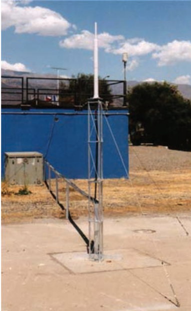
Fig. 5.9: DORIS antenna (standard layout 2 m tower), from Fagard (2006).
