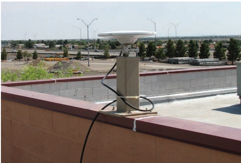
Fig. 7.15: CORS station equipped with a Trimple Zephyr Geodetic Antenna, El Paso, TX, U.S.A., courtesy NGS ( http://www.ngs.noaa.gov/CORS ).
