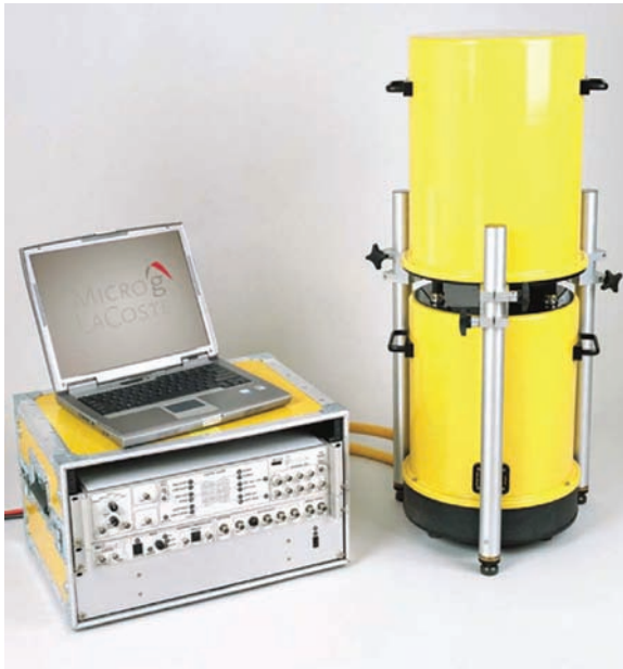
Fig. 5.56: Portable absolute gravimeter A-10, courtesy Micro-g LaCoste – A Division of LRS, Lafayette, CO, U.S.A.
