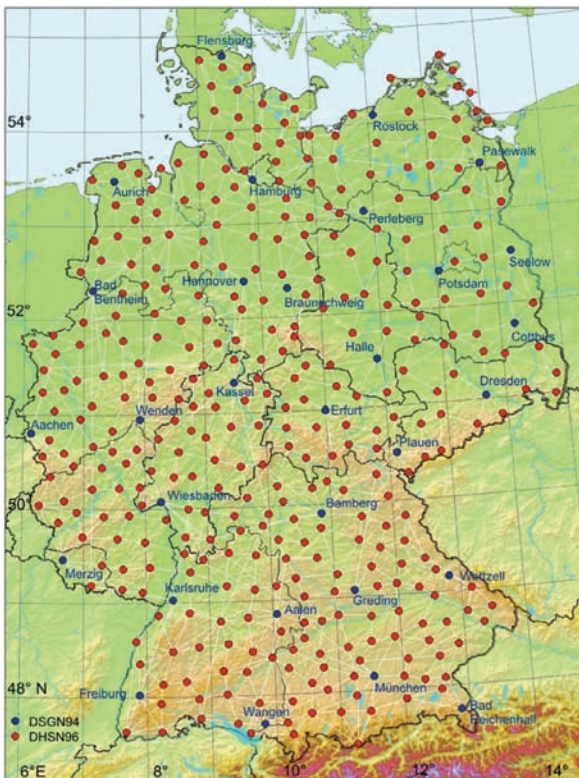
Fig. 7.22: Primary gravity net (red circles) of Germany (DHSN96), with German gravity base net (DSGN94) stations (blue circles), courtesy BKG, Frankfurt a.M., Germany.
