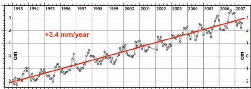
Fig. 8.18: Sea level rise between 1993 and 2007 (monthly mean Values), derived from TOPEX and Jason1 satellite altimetry, after Bosch et al. (2010).
