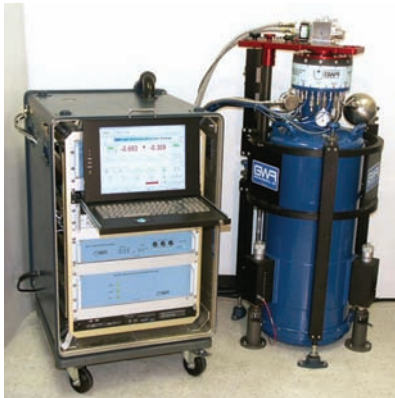
Fig. 5.75: OSG Observatory Superconducting Gravimeter view, courtesy of GWR-Instruments Inc., San Diego, CA, U.S.A.
