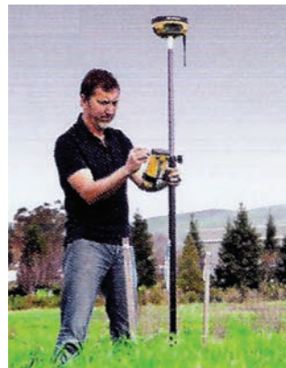
Fig. 5.18: GPS/GLONASS rover TOPCON HiPer II, courtesy TOPCON Europe B.V., Capelle a/d IJssel, Netherlands.
