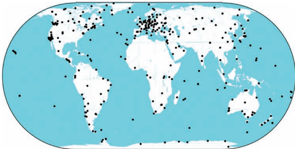
Fig. 5.20: Network stations of the International GNSS Service IGS (status 2010), courtesy IGS ( http://igsceb.jpl.nasa.gov/ ).
