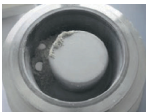
Fig. 3. Preparation of routine cement sample: 45 g of the sample is poured into a 50 ml WC jar and 2 \times 0.25 g tablets of FLUXANA Multimix are added. A 40-mm pellet is produced by pressing at 25 tons
