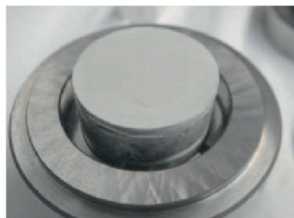
Fig. 4. Preparation of calibration standard with wax: 6 g of the powder is mixed with 2 g of FLUXANA wax. A 40-mm pellet is produced by pressing at 25 tons
