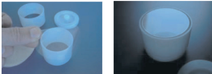
Fig. 1. Preparation of a liquid cell or sample cup for the direct analysis of powders or liquids
