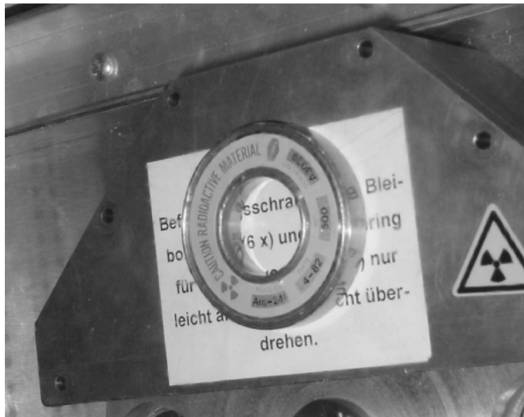
Fig. 2.28. The photo of a 241 Am-ringshaped XRF-source [12]
