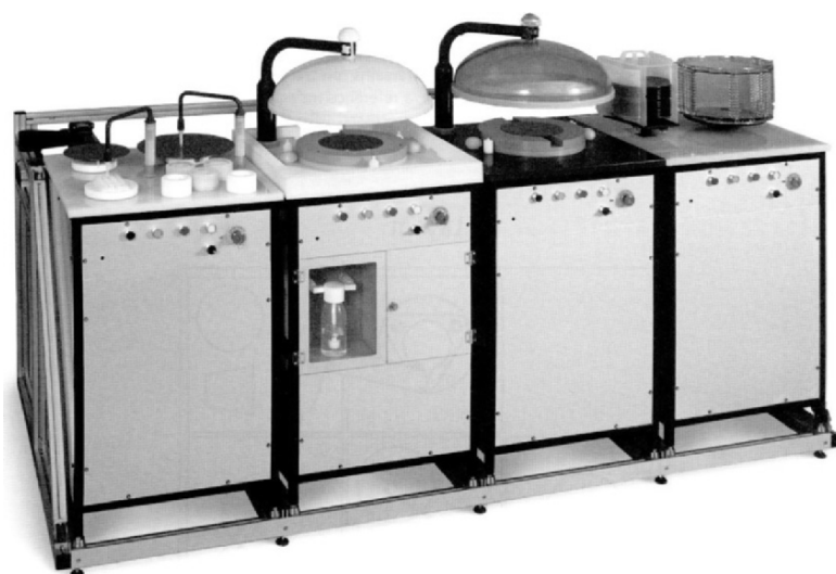
Fig. 7.50. Wafer surface preparation system modules (WSPS): a novel system for vapor phase decomposition preparation for wafer diameters 100 up to 300 mm
