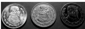
Fig. 7.151. The obverse of the silver plated Mexican Pesos; from left to right increasing wear off of the surface layer as determined by the XRF investigation depicted in Fig. 7.150
