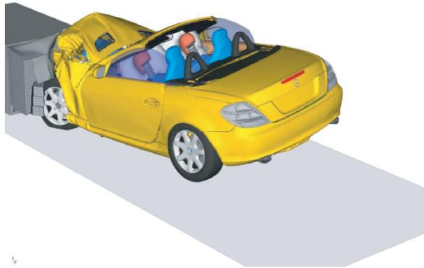
**Fig. 1.4.** Crash of a car against a deformable barrier, from Daimler Chrysler AG.
