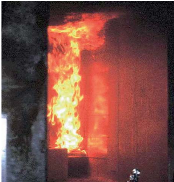
Figure 11.13. Room corner test. Photograph supplied courtesy of the CRC for Advanced Composite Structures Ltd.
