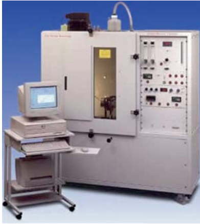
Figure 11.9. General view and schematic diagram of the N.B.S. smoke chamber. The photograph and diagram is reproduced with permission from Fire Testing Technology Ltd. and Greene [25], respectively.
