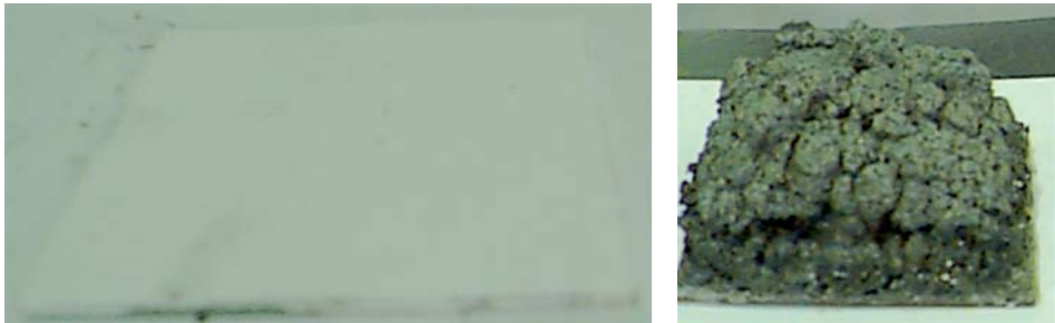
(a) (b) Figure 8.27. Intumescent coating (a) before fire testing (thickness = 0.8 mm) and (b) after fire testing (thickness = 52 mm). Photographs supplied courtesy of Z. Mathys (DSTO).
