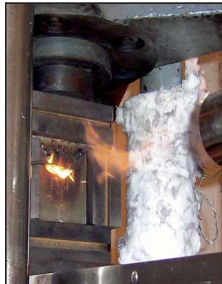
Figure 6.16. Restrained compression test. (a) Schematic of picture frame restraint jig and (b) propane burner test on a polymer laminate under compression.
