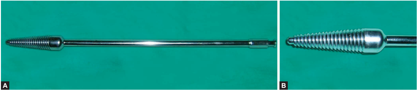
Figs 13.26A and B: Leech Wilkinson's cannula: (A) The whole equipment; (B) Tip of Leech Wilkinson's cannula
