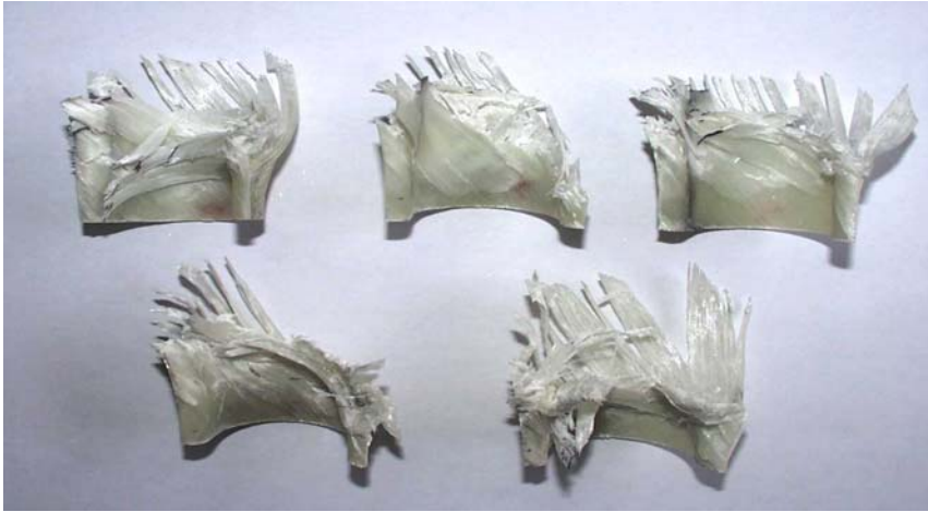
Figure 3. Energy absorption structure failure modes.
