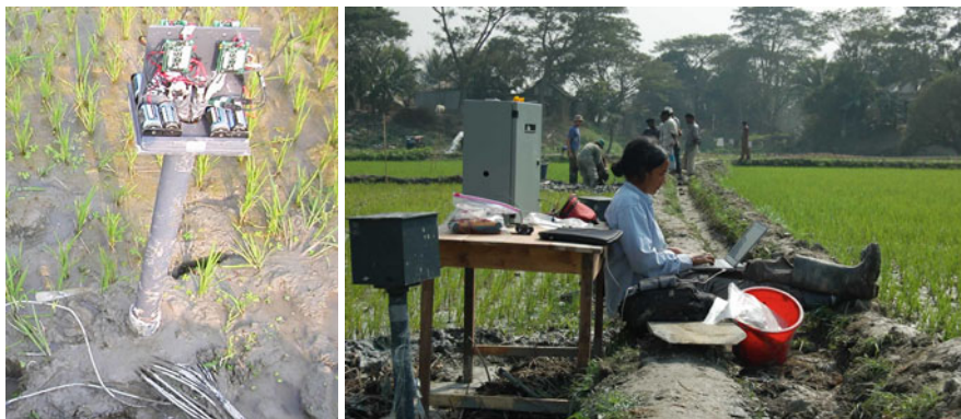
Fig. 2.1 Photos from the deployment site in Bangladesh. The photo on the left shows a sensor node with the case open. The photo on the right shows part of the deployment process. The large metal cabinet houses the base-station and data collection server. Original images used with permission of Charlie Harvey, MIT Civil and Environmental Engineering
