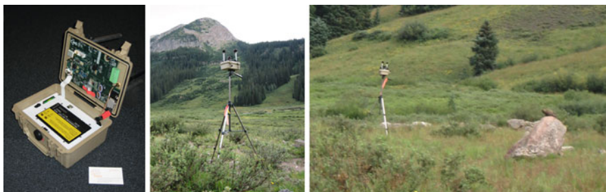
Fig. 2.4 The VoxNet System. From left to right : the node hardware with the case open, showing the sensor interface board (the CPU modules are under the battery); one of the nodes, deployed in Colorado, USA in 2007; a VoxNet node locating a marmot. Original images used with permission of Lewis Girod, MIT/CSAIL
