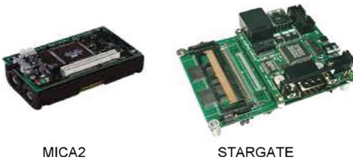
Fig. 7.7 Mica2 and Stargate [17] used with permission copyright ACM 2009
