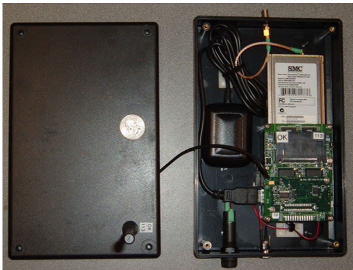
Fig. 8.2 The eXtreme Scale Stargate. Each XSS has an Intel 400 MHz XScale R processor (PXA255) with 64 MB SDRAM, 32 MB FLASH, type II PCMCIA slot, USB port, and 51-pin mote connector; packaging is watertight. Original Figure used with permission of IEEE [23]
