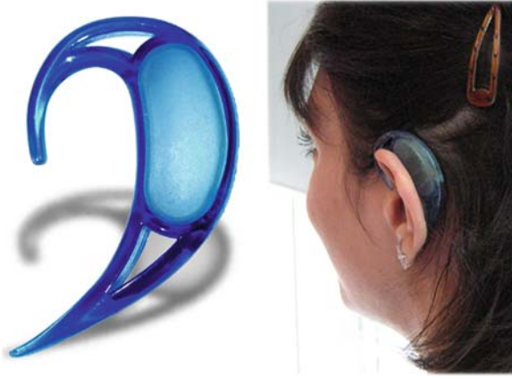
Fig. 2 The e-AR sensor developed at Imperial College London comprises a Nordic nRF24E1 chipset, built-in 2.4GHz RF transceiver, memory, and an analog-digital converter for data sensed using a 3-axis accelerometer. This is based upon a miniaturised design of the BSN node [65]
