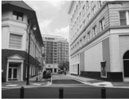
Figure 2.8: My photograph of a closed-in street in downtown Durham depicts a small skyview factor — the small patch of viewable sky versus all the walls blocking a larger skyview. This skyview factor (0 means no viewable sky, and 1 means a fully open sky) resolves the North American–European difference seen in Figure 2.7. Plotting a city’s urban heat island effect against its skyview factor, instead of its population, results in a single curve for all three regions plotted here (after Oke 1982). Evidently, large European cities possess shorter buildings with more open-sky views.
