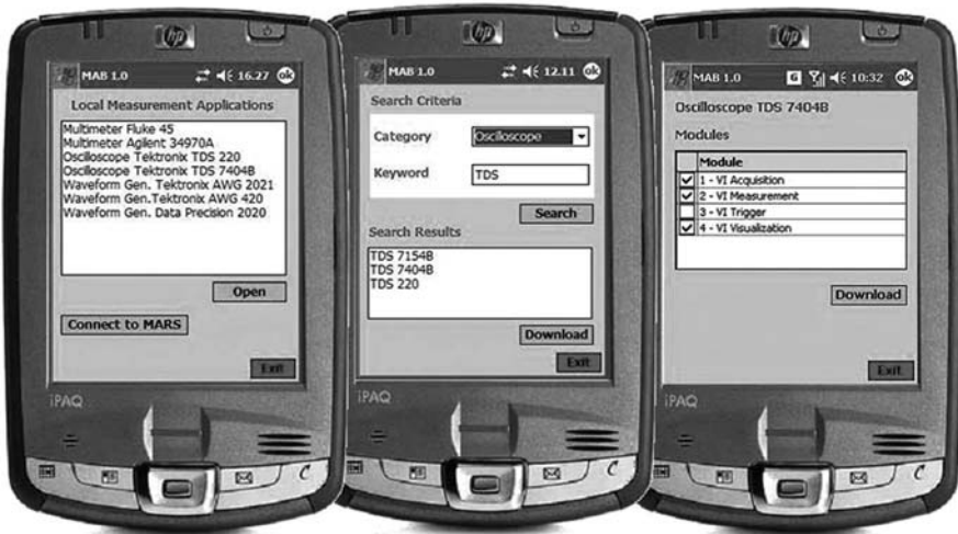
Fig. 35.4 Experiment creation on PDA. From left to right: (a) available applications, (b) search application, and (c) modules of each application
