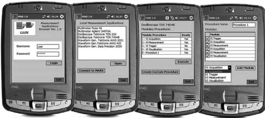
Fig. 35.3 Experiment creation on PDA. From left to right: (a) login, (b) available applications, (c) modules of each application, and (d) list of available modules
