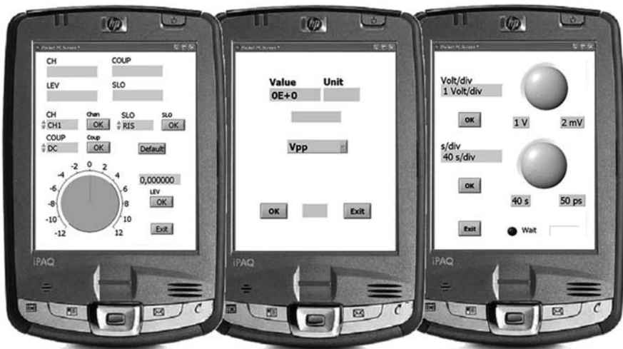
Fig. 35.5 GUI of each downloaded module. From left to right: (a) trigger module, (b) measurement module, and (c) acquisition module
