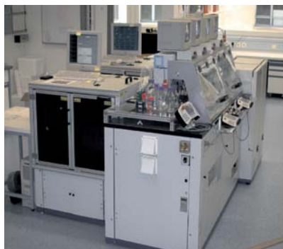
Fig. 13. The Evotec Mark II SCARINA (screening and readout in NanoCarriers) compound testing and plate handling NanoScreen system. The system can handle both 1,536w- and 2,080w-NanoCarrier plates and is equipped with four reagent dispensing tables and with two fully automated confocal fluorescence microscopes for detection. Compound storage devices, plate handling devices, and system control are integrated into one screening station
