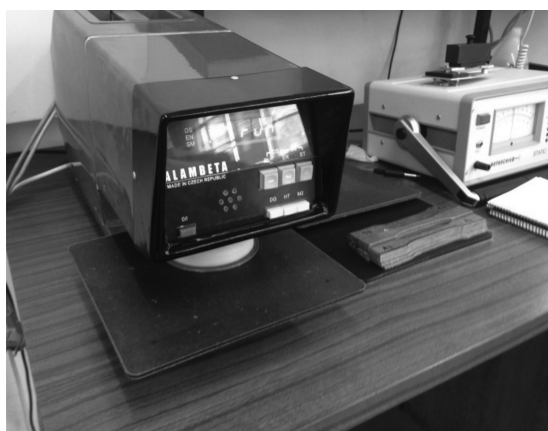
Figure 5. Alambeta device and analytical balance for thermal and moisture absorption tests, respectively.
