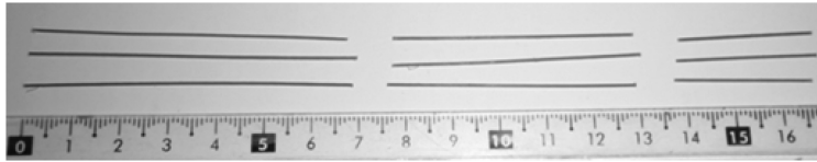
Figure 1. Synthetic waste fibres used in the concrete mix.
