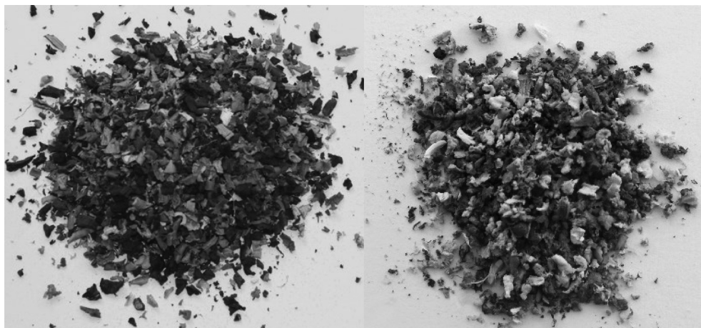
Figure 1. Waste with particle size bigger than 2 mm and smaller than 1 mm, respectively.
