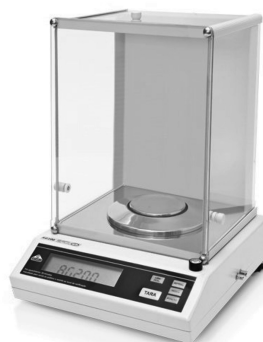
Figure 5. Alambeta device and analytical balance for thermal and moisture absorption tests, respectively.
