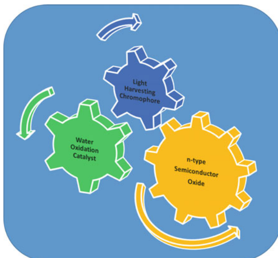
Fig. 6.2 Conceptual design of the key elements of a photoanode in a light-driven, water-splitting photoanode
