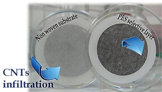
Figure 5.15. The infiltration process carried out by filtering a CNT-suspension from the support side (left) to reach the selective layer (right). The black imprint of CNTs on the side of the selective layer is clearly indicating their existence to the surface pores, while the substrate is empty of CNTs, indicating that all CNTs were pushed towards the PES skin layer.
