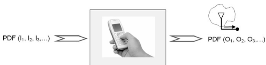
Fig. 4.33 Schematic view of the input–output relation between the statistics of input (parameters defining the terminal) and output (antenna characteristics) random variables for an antenna system
