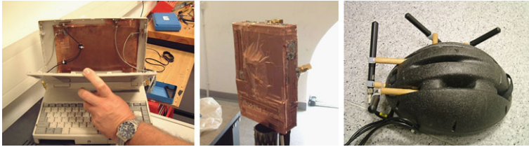
Fig. 4.5 Realistic and reference antenna configurations for evaluation of eigen coherence time [BHW07] (©2007 EurAAP, reproduced with permission)
