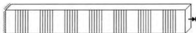
(d) specimens CJS & GJS, with one layer fibre, three sides of the section (U-jacket), 7 strips of 100mm spaced at 100mm.
