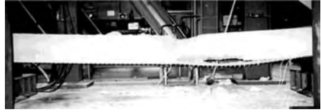
Figure 3. Failure of 3.7 m beam with MF-FRP strip.
