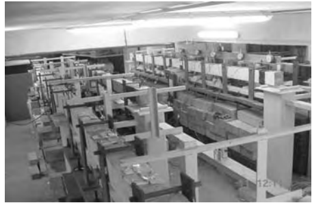
Figure 3. Test set-up for glass FRP-bonded RC beams.
