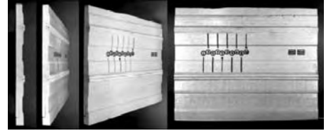
Figure 2. CE specimen with thermocouples slots.
