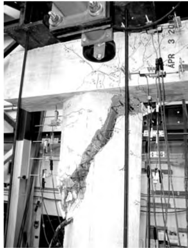
Figure 6. Shear failure in the south column of the as-built specimen.
