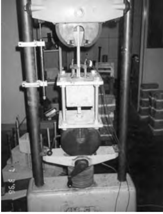
Figure 13. Pull-out test arrangement.
