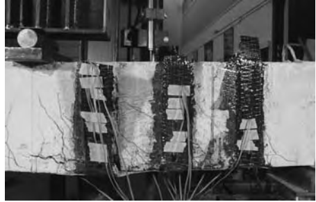
Figure 8. Failure of beam A1b.
