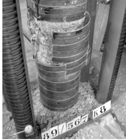
Figure 1a. Failure of HFRP fully wrapped column.
