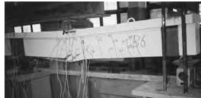
Figure 5. Typical peeling failure of the strengthened beams.
