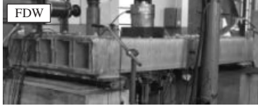
(b) FRP deck with outside filament winding
