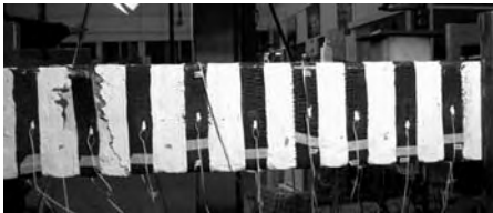
Figure 8. CFRP rupture in Beam F2.
