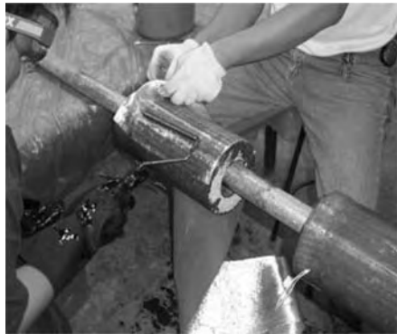
Figure 3. Formation of the FRP tube.
