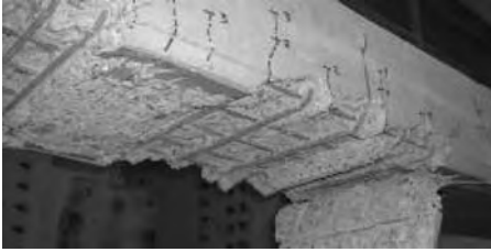
Figure 3. Development of crack in correspondence of stirrups.
