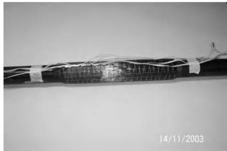
Figure 3(c). Typical specimen with strain gages.
