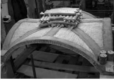
Figure 5. FRP strengthening of a masonry cross vault.
