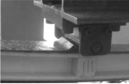
Figure 3. Compressive failure and debonding of the upper CFRP plate.
