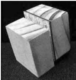
Figure 4. Typical failed shear cube sample.
