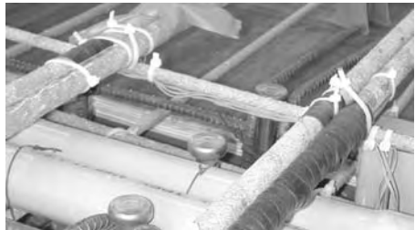
Figure 12. Protected sensors complete with properly located and secured lead wires.
