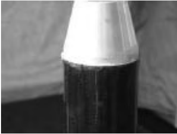
(c) Debonding failure under compression
