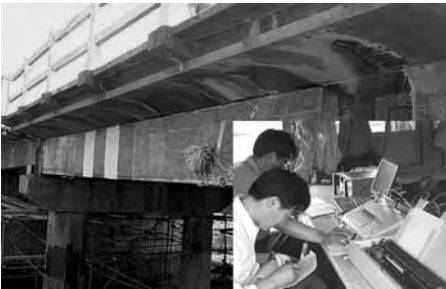
Figure 8. Data acquisition and monitoring post-strengthening performance of the bridge span (Jamaji et al. 2003).
