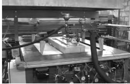
Figure 8. Setup for liquid cooling (LC) experiments.
