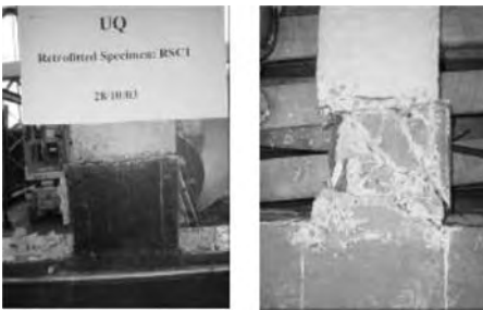
Figure 8. Failure pattern of specimen RSC1.
