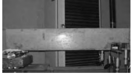
Figure 2. Photograph of dowel test setup.
