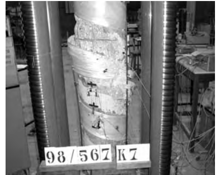
Figure 1b. Failure of GFRP partially wrapped column.
