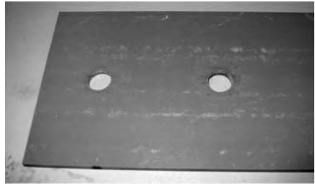
Figure 8. Slip wear marks on the inner 9.53 mm thick PFRP plate.
