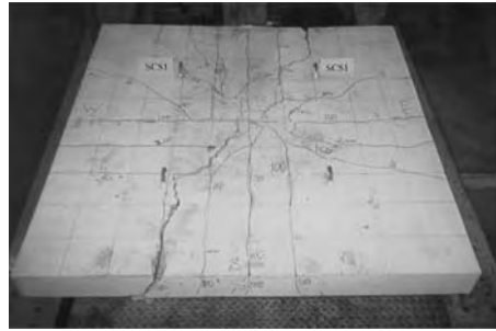
Figure 11. Shear fracture surface of slab SCS1 after failure.
