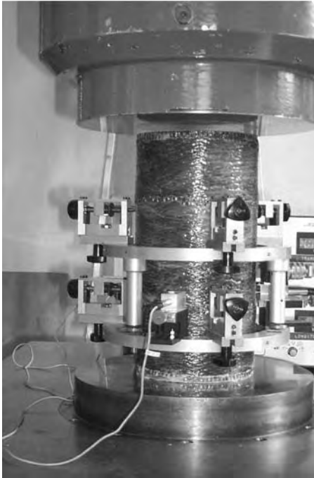
Figure 1. 16 × 32 retrofitted concrete sample during test.
