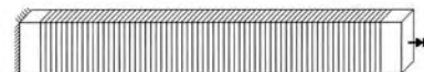
(e) specimens CJE & GJE, with one layer fibre, three sides of the section (U-jacket), along the entire beam.
