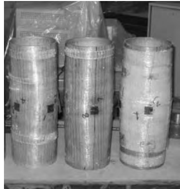
Figure 6. FRP-confined steel tubes after compression test.
