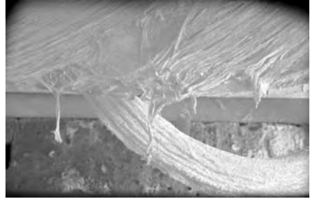
Figure 9. Reinforcing roving layers drooping down and oxidizing (LC experiment).
