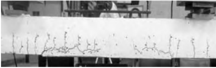
Figure 7. PE debonding in constant moment region.
