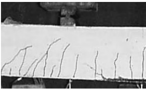
(a) Cracking patterns of beam A2
