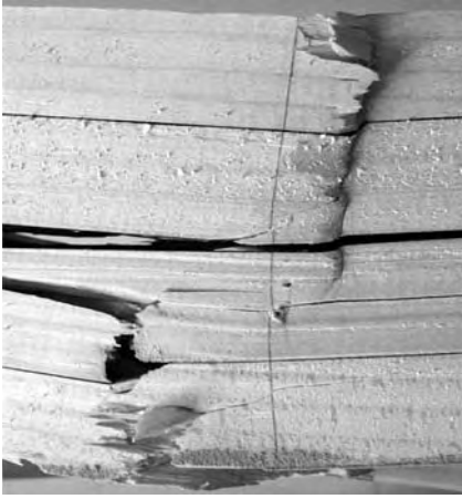
Figure 8. Initial compression failure in upper laminates followed by tensile failure in lower laminates.
