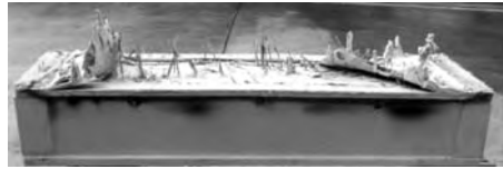
Figure 10. Post-fire hot face of LC03 specimen.
