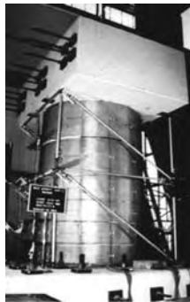
Figure 4. Cyclic load test on the same full scale bridge pier strengthened with FRP. Specimen shows no cracking of the RC pier (Fyfe 2001).
