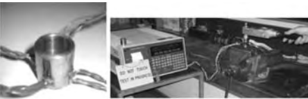
Figure 3. (a) Bolt tension load cell. (b) Set-up for calibration.
