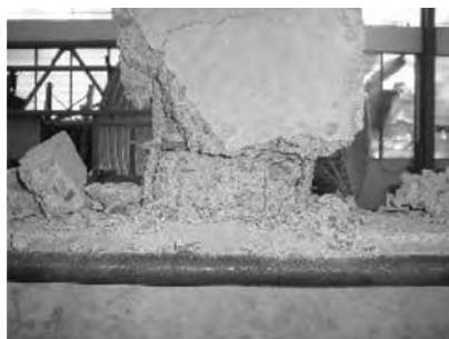
Figure 5. Failure pattern of specimen CSC1.
