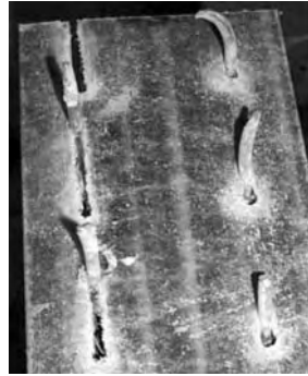
Figure 12. Shear-out failure at end of strip in A3-1.
