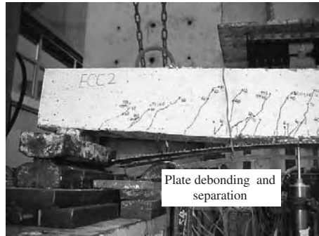
Figure 5. Debonding and separation of CFRP in beam ECC-2.
