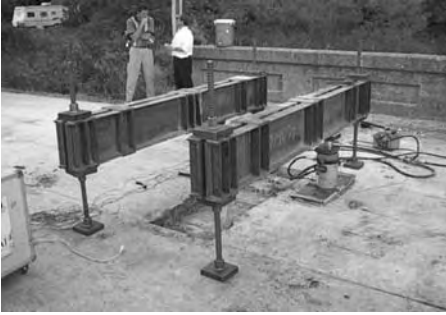
Figure 19. Failure load testing of the MF-FRP strengthened bridge.
