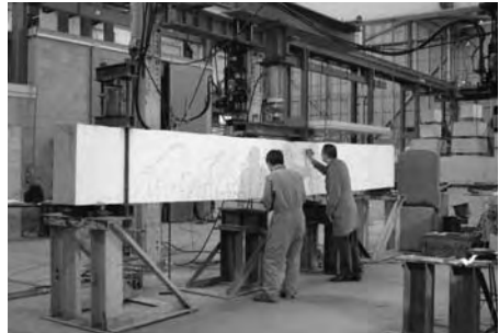
Figure 12. Beam B2 after debonding failure.
