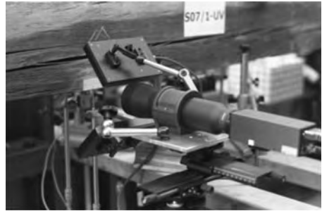
Figure 6. Photogrammetric measurement of deflections.
