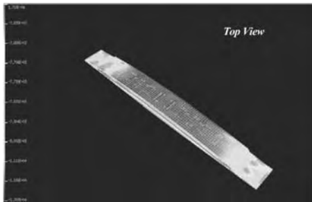
Figure 15. Generalized normal stress N_x distribution after 128,140 cycles ( Fatigue Life ) – top view.
