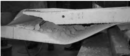
Figure 9. a) Failed Hebel AAC Powerpanel – externally reinforced. b) Failed Hebel AAC Powerpanel – externally reinforced (close view of failure).
