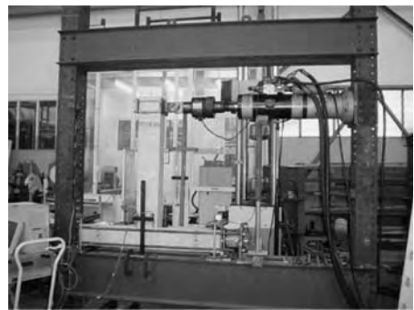
Figure 1. Beam-column joint testing set-up.
