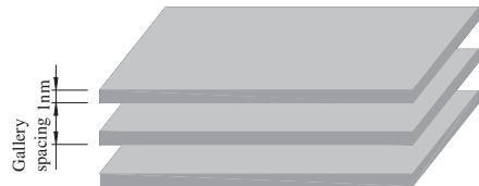
Figure 3. Structural representation of smectite clay layers.
