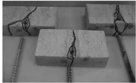
Figure 14. Crack patterns for some of the tested specimens.
