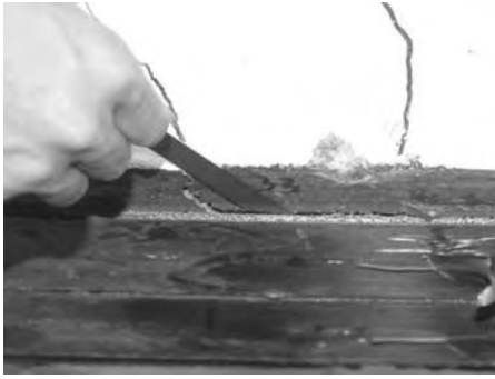
Figure 13. Initiation of intermediate debonding failure (B6 at P = 450 kN).
