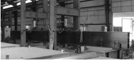
Figure 2. Four-point bend test set-up for 91 cm (36 inch) DWB.
