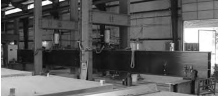
Figure 2. Four-point bend test set-up for 36 inch DWB.
