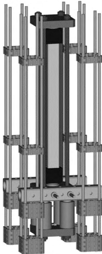
Figure 6. Strengthened RC column test equipment.
