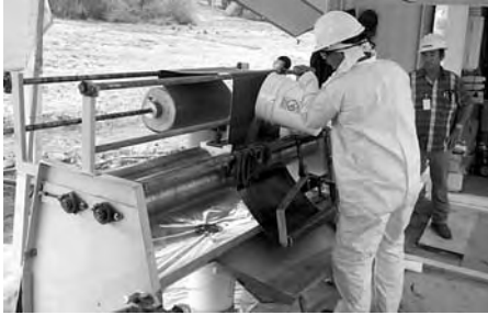
Figure 9. A mechanical fabric saturator to control the fibre-resin ratio in operation (Fyfe 2001).
