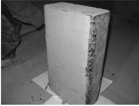
Figure 3. Primer and putty application.
