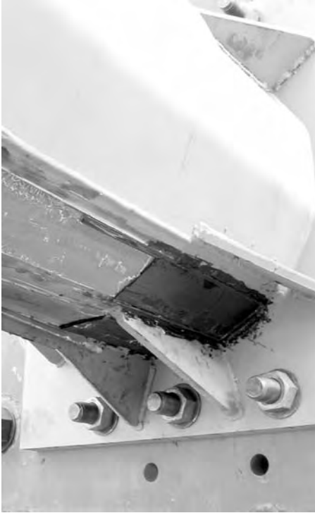
Figure 8. Rupture of CFRP strips at end of gusset plates for monopole (MAB-H).
