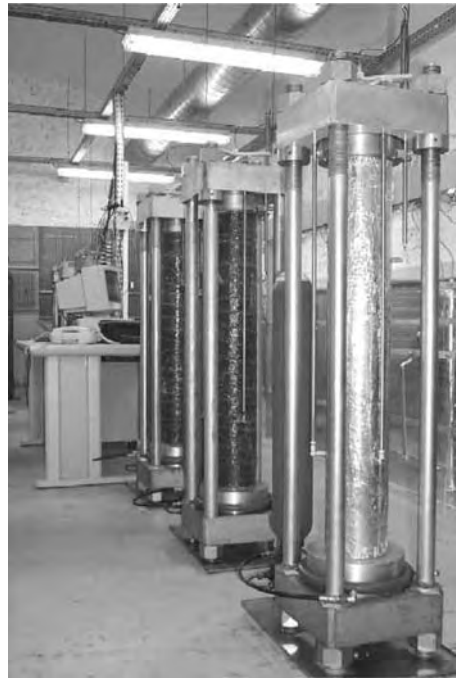
Figure 3. Strengthened concrete samples and reference concrete sample under creep loading (20°C, 50% RH).
