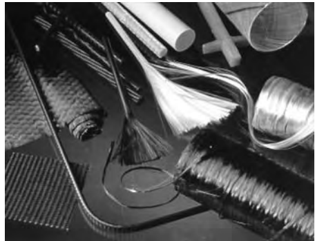
Figure 1. A variety of FRP products used in ISIS Canada research and applications.
