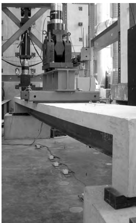
Figure 11. Test setup for steel–concrete composite beam (CGAB-I) before strengthening.
