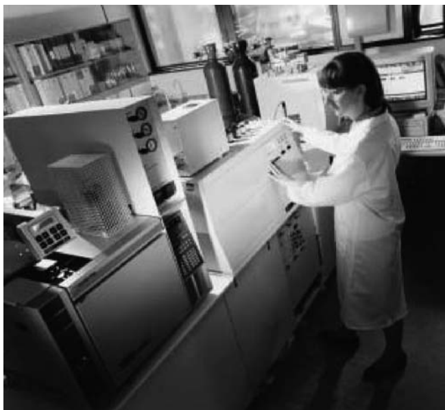
Fig. 1 Gas chromatography combustion isotope ratio mass spectrometry for assay of aqueous ethanol calibration standards. This method offers lower uncertainty than the previous titrimetric procedure and may also be used directly to obtain ethanol reference values in alcoholic beverages
