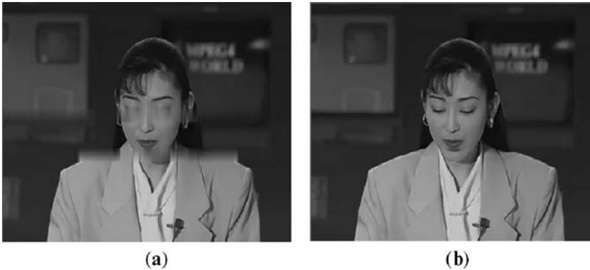
Fig. 16.7 Comparison between the result of (a) the Error Concealment algorithm in JM7.3 and (b) its modified version, for frame #60 of the Akiyo sequence
