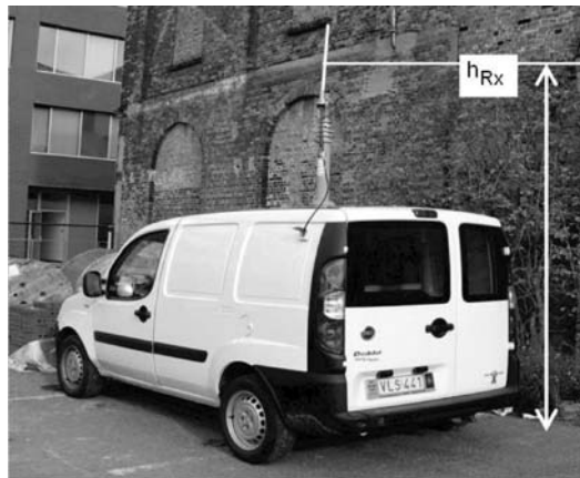
Fig. 1.6 Vehicle with Rx used for the data acquisition
