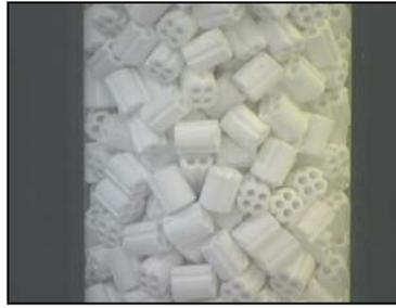
*Figure 10.* Tube Packed with Reforming Catalyst
