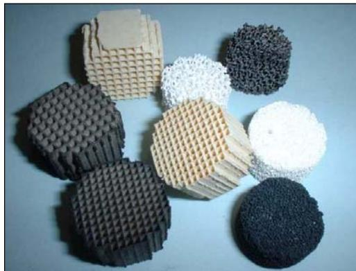
Figure 1. Structured honeycomb and foam catalysts based on supported  $\text{LaMnO}_3$  perovskite for high temperature oxidation processes.
