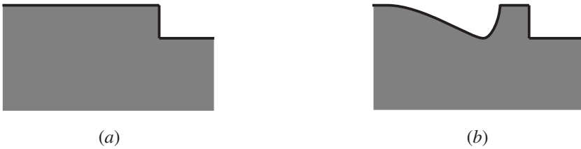
Figure 6-8: Guiding the lines of stress by means of notches that are not functionally essential is a useful method of reducing the detrimental effects of notches that cannot be avoided. These are termed relief notches. It is assumed here that the bearing surface of the step of (a) is needed functionally. Adding a notch as in (b) can reduce the hazardous effects of the corner of (a).
