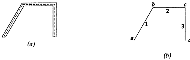
Figure III-26: Simple plane frame: (a) framework; (b) model with elements (bars) 1, 2, 3 and nodes (joints) a, b, c, d.
