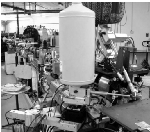
Figure 3 : View of the external nuclear microprobe beam line of the“AGLAE” accelerator. © C2RMF.
