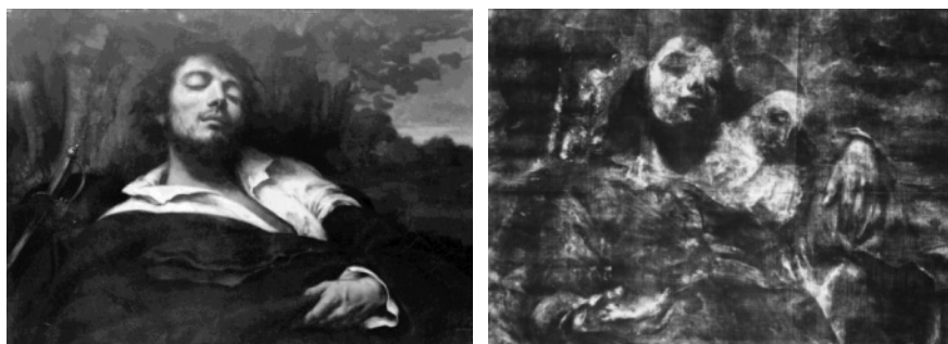
Figure 1. The radiography of “L’homme blessé” by Gustave Courbet , 1844 – 1854, 815 x 975 mm, Musée d’Orsay, Paris reveals two previous compositions. Left figure: visible image, right figure : radiography. © C2RMF.
