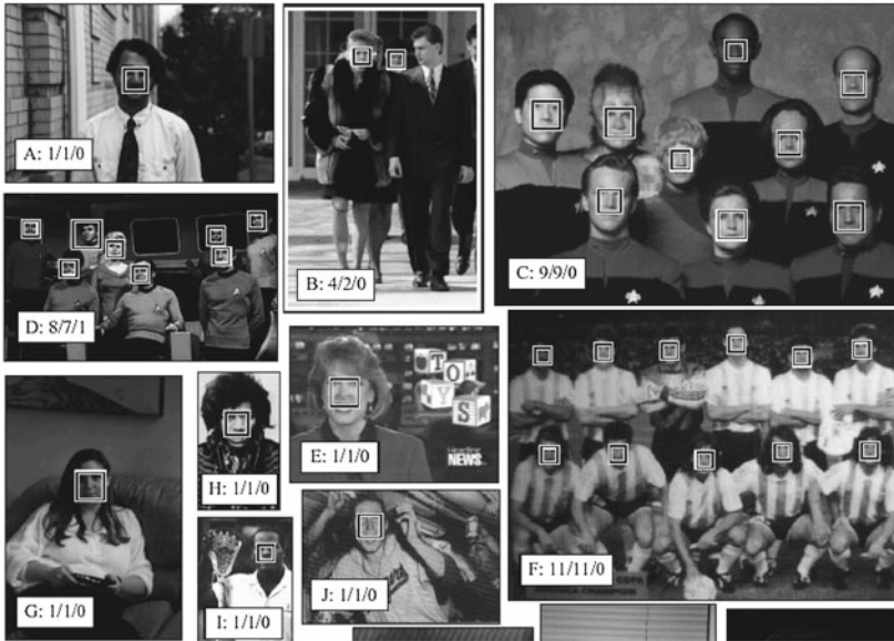
Fig. 7.2 Face detection using neural network-based method (Rowley et al. 1998). © 1998, IEEE. Reproduced with permission
