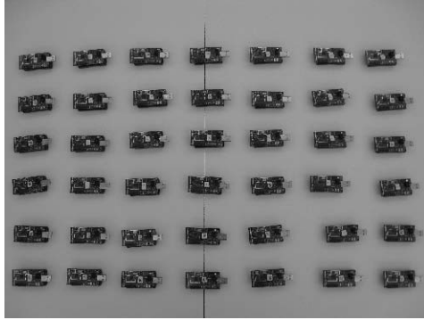
Figure 5.10: Layout of 42 X-bow T-Sky Motes.
