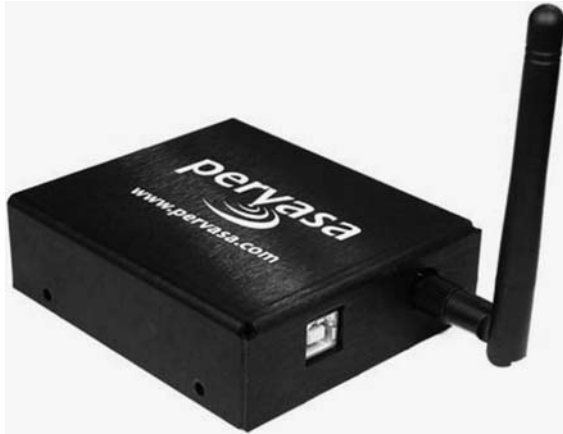
Figure 16. Atlas ZigBee node in ruggedized packaged form factor.
