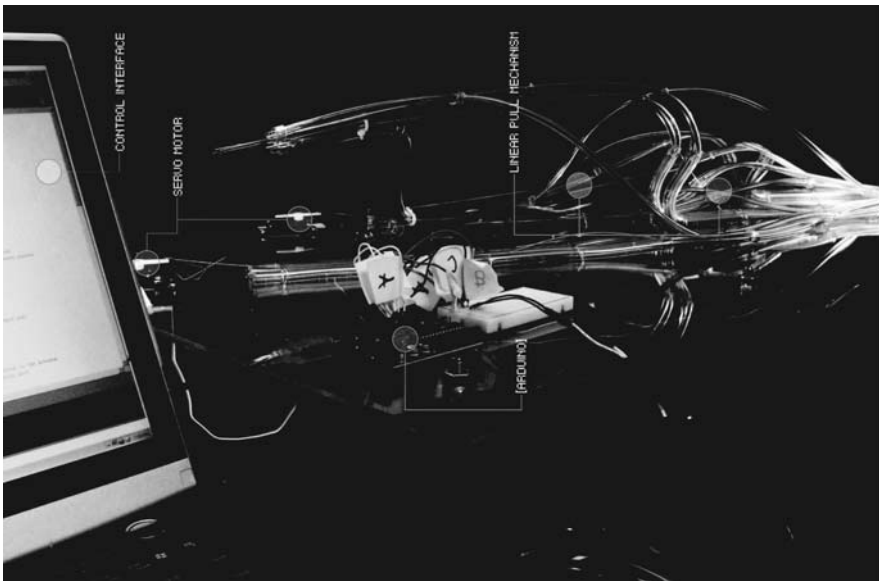
Figure 10. Robotic prototype 2CELLv.2 actuated with an Arduino micro-controller via an interface developed in Max/MSP.
