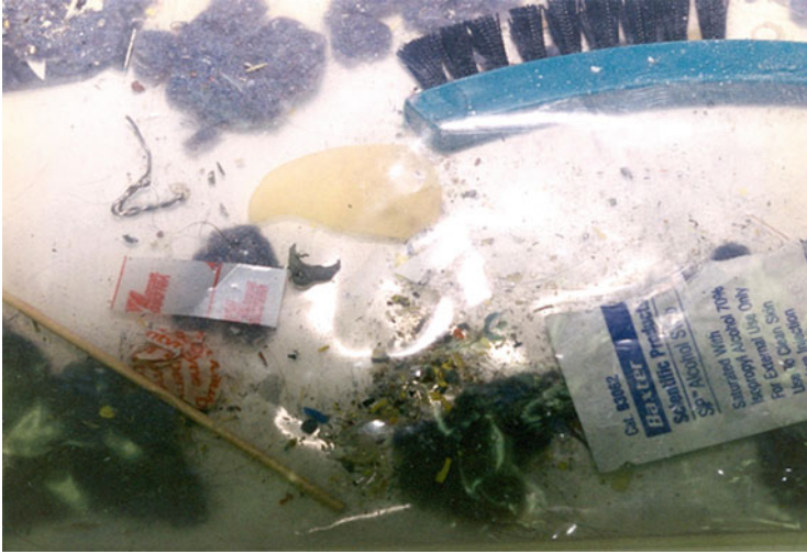
Fig. 1.3 Debris collected on air filters in Spacelab module in the Space Shuttle. Note large debris including small bristle brush, wooden stick, and various paper wrappers
