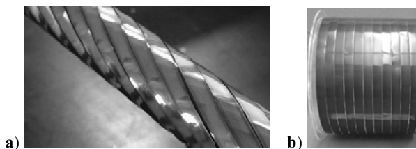
Fig. 15. a) The first 2 nd generation demonstration cable (made by Southwire, from American Superconductor) uses second generation \text{YBa}_2\text{Cu}_3\text{O}_7 tape conductor prepared by RABiTS technique, tested by Oak Ridge National Lab.: I_{dc} \sim 4.2 kA at 77 K, 1.25m length, 24 total tapes, 50 \mu\text{m} of copper stabilizer (courtesy of American Superconductor); b) \text{YBa}_2\text{Cu}_3\text{O}_7 film was deposited by the PLD method on the biaxially textured Ag-Cu/Ag-Ni/Ag-Cu clad tape, substrates exhibits (110) \langle 220 \rangle texture uniformly throughout the whole length, shows the uniform current distribution, J_c > 10^5 \text{Acm}^{-2} , in the 10 m-long tape, coil diameter 25cm [46]. Courtesy of Y. Shiohara.
