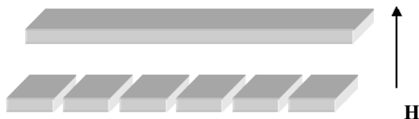
Fig. 35. Schematic of the fragment of the single filament and multifilamentary coating in external magnetic field.
