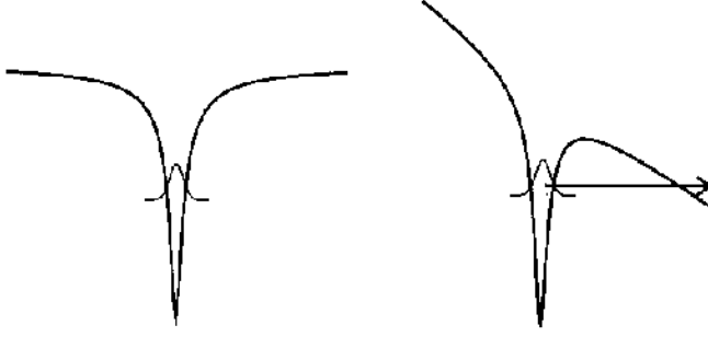
Fig. 12.3. Schematic of the potential created by the ionic core only (left) and by the strong field + ionic core (right). When the field is strong enough, the electron can escape the core attraction and reach the continuum by tunneling through the potential barrier
