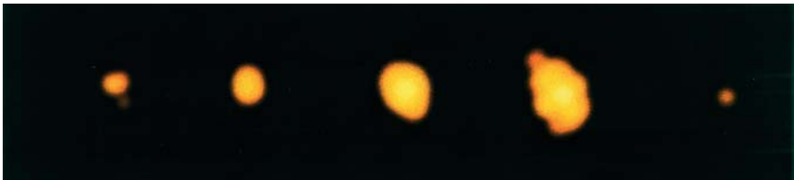
Fig. 8.42. Diffraction pattern observed on the screen in the setup shown in Fig. 8.41. Left to right: second order, first order, pulse 1, pulse 2, first order
