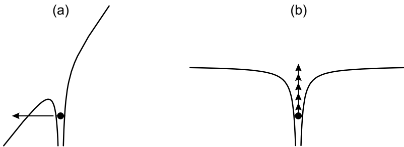
Fig. 5.9. Illustration of ionization of atoms via (a) electrostatic tunneling at large laser fields (Keldysh parameter \gamma_K \ll 1 ) and (b) multiphoton absorption at weak laser electric fields ( \gamma_K \gg 1 ). According to Example 5.1, \gamma_K = 1 corresponds to a laser intensity of 10^{14} W/cm 2 for typical parameters [267].
