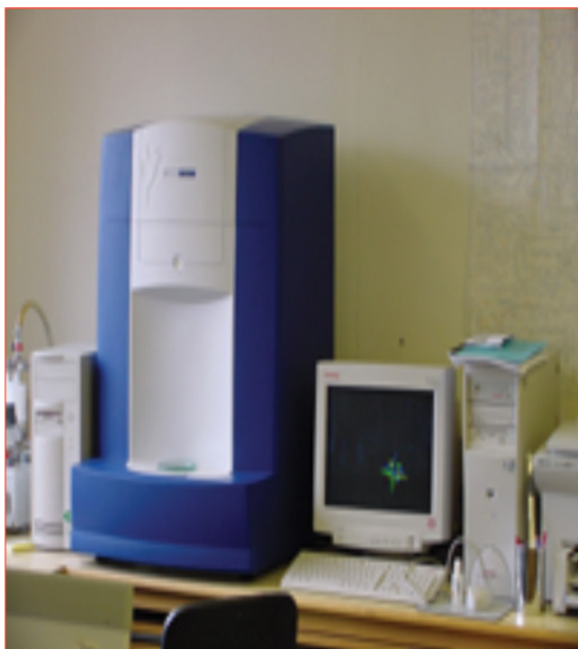
Figure 1.5 The first dedicated linear MALDI-TOF mass spectrometer for microbial identification used for creating the first MALDI-TOF MS database in 2004 (Keys et al. , 2004). The instrument, manufactured by Micromass (Manchester, UK), remedied many of the shortcomings of the Kratos Kompact Alpha and had the capacity to analyze 96 samples automatically.
