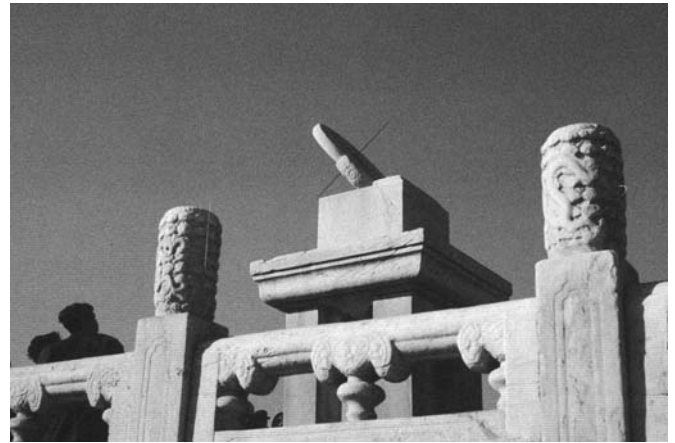
FIGURE 4.6. A stone equatorial sundial in the Forbidden City in Beijing, China: The dial disk lies in the plane of the celestial equator and thus faces the north celestial pole. Photo by E.F. Milone.
