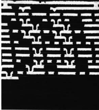
Fig. 11.36. Cross-section through a completed multilayer printed circuit board for the Siemens 7500H90 computer produced with a KrF excimer laser [4]
