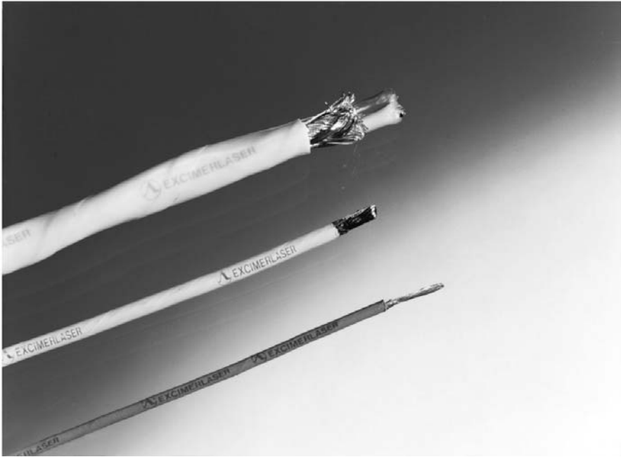
Fig. 16.16. Marking of Teflon ® -coated wires with 308 nm radiation
