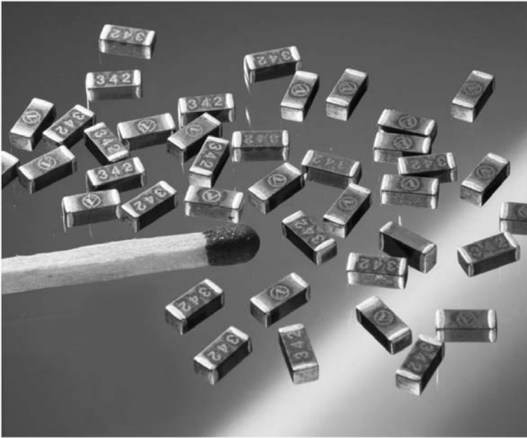
Fig. 16.18. Marking of surface mounted devices (SMDs) [7]
