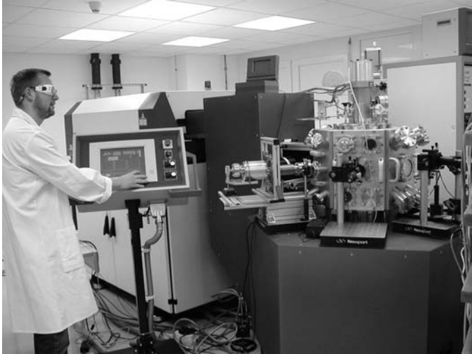
Fig. 22.5. LPP laboratory EUV source at XTREME technologies. The 500 \text{ W} diode-pumped solid-state laser (left side) excites the target in the vacuum interaction chamber (right side).
