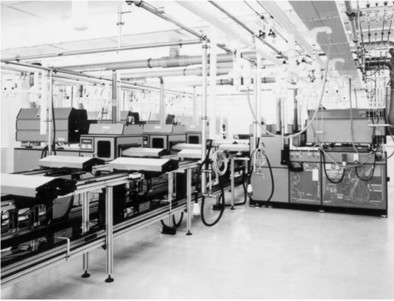
Fig. 1.10. Large industrial excimer installation at Siemens Nixdorf Informationssysteme, Augsburg, Germany, containing 9 EMG 1003i excimer lasers in 1988
