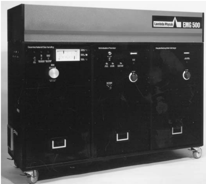
Fig. 1.6. The first commercial multigas excimer laser EMG 500. Pulse energy of 220\text{ mJ} @ 248\text{ nm} , repetition rate between 0.05\text{ Hz} and 20\text{ Hz} .
