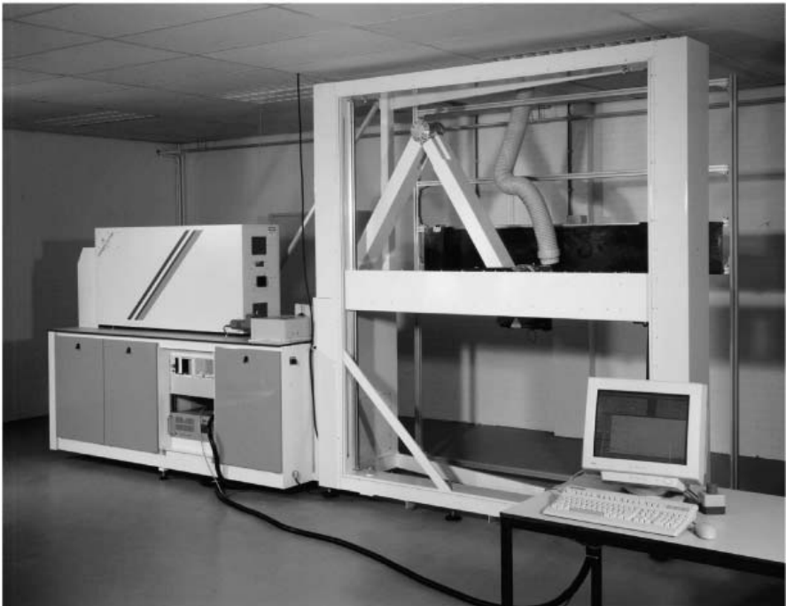
Fig. 10.2. Laser cleaning workstation consisting of Lambda Physik COMPEX 205, LIBS detection system and beam steering and suction device for the restoration of works of art; by courtesy of Art-Innovation b.v., Hengelo, The Netherlands
