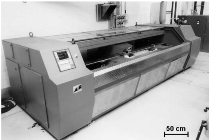
Fig. 11.6. Prototype installation for the cleaning of rotogravure cylinders; by courtesy of ILT
