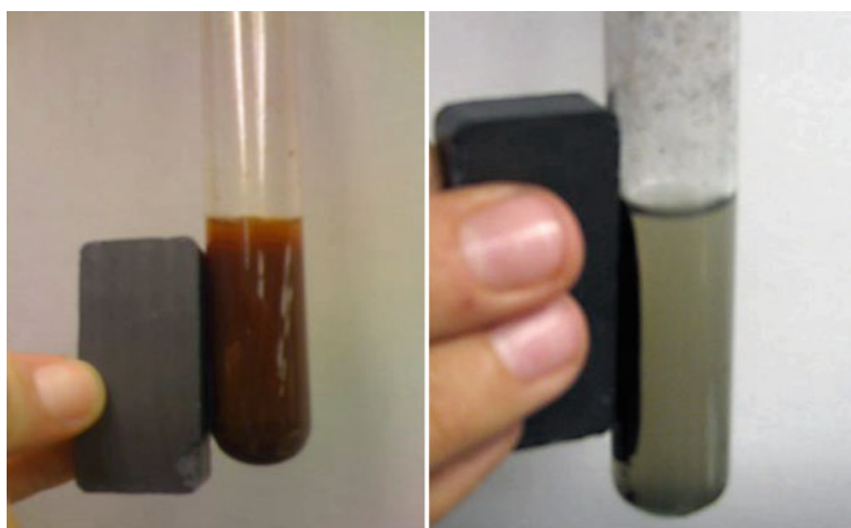
Fig. 2 Iron in the culturing medium that has been converted into magnetite will be attracted by a magnet through the wall of the culturing tube (Photo credit: J. Cameron Thrash. Hand model: Kelly Wrighton)
